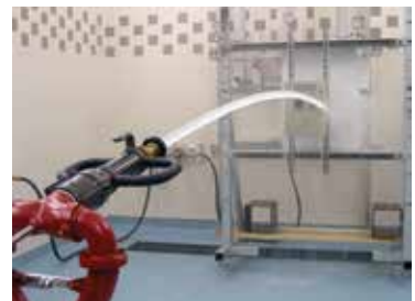
iQpump Micro NEMA-4X Washdown Test
