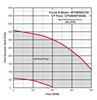
Total Dynamic Head is equal to vertical lift, maximum operating pressure and friction loss. These curves are for general guidance only, individual curves are available upon request. A certified curve may be requested for an additional cost. Webtrol will build pumps to fit your specific needs, contact factory for pricing.
