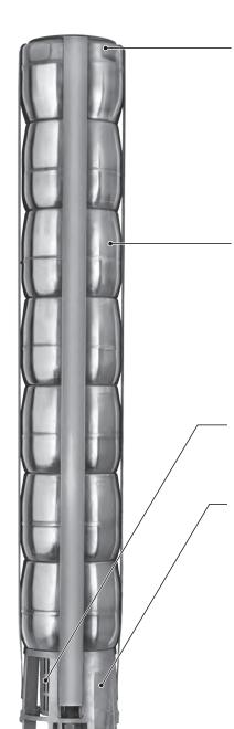
**Discharge Head:** Precision stamped and welded 304 stainless steel discharge head\* provides a smooth flow transition with a minimum amount of restriction. Includes a built in, jam free, stainless steel check valve to prevent back flow of water.
